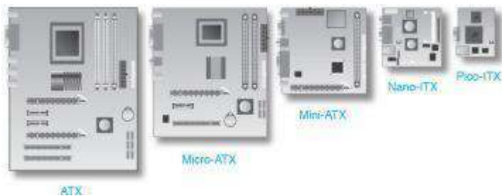
Figure 3.39 Motherboard form factors
